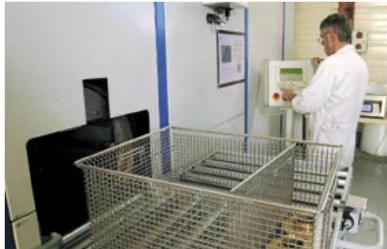
The system continuously re-treats the cleaning agent via an integrated vacuum distillation, water separation and residual distillation unit that limits consumption while guaranteeing efficiency.
