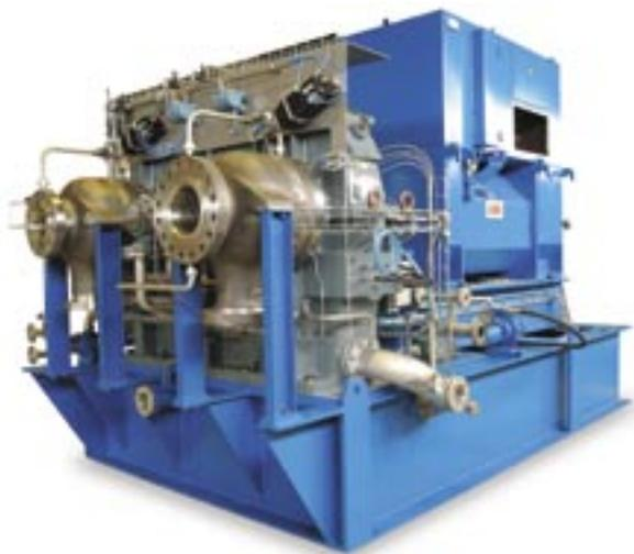
Such ER-units utilise the potential energy of natural gas being delivered under high-pressure. The gas is only expanded when it reaches the pressure let down station, and it is here ER-units come into their own.
