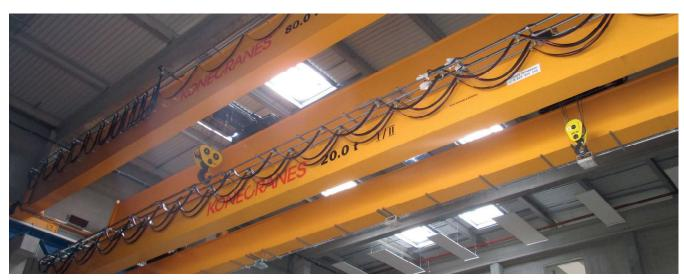
The 4 cranes were delivered and installed in March 2022. Each of the two halls is equipped with an 80t and a 20t crane.
