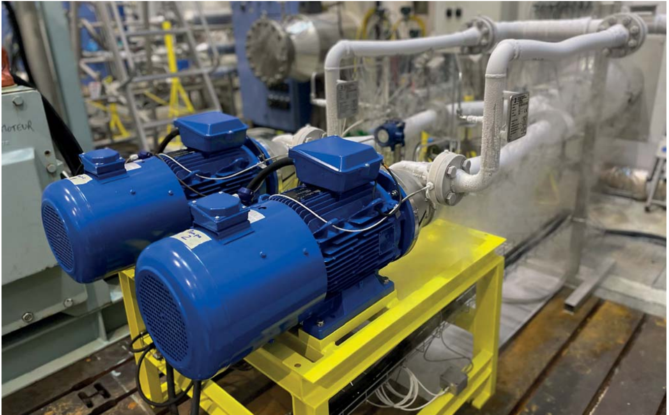
2 GBS pumps undergoing an endurance test
