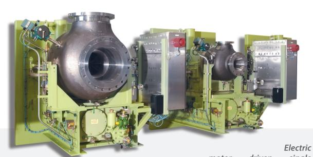
motor driven single stage cryogenic compressor, type CM, with adjustable inlet guide vanes, complete with lube oil system, seal gas system, and accessories. The whole unit is installed on a single, rigid skid, with bulkhead, and bulkhead seal mounted to the heavy-duty gearbox. Capacities of up to 40'000 m3/h of boil-off gas with an inlet temperature of -140 degC are available.
