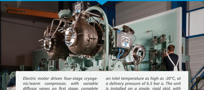
nic/warm compressor, with variable diffusor vanes on first stage, complete with lube oil system, seal gas system, and accessories. Typically this machine delivers up to 5'500 m3/h of boil-off gas with
