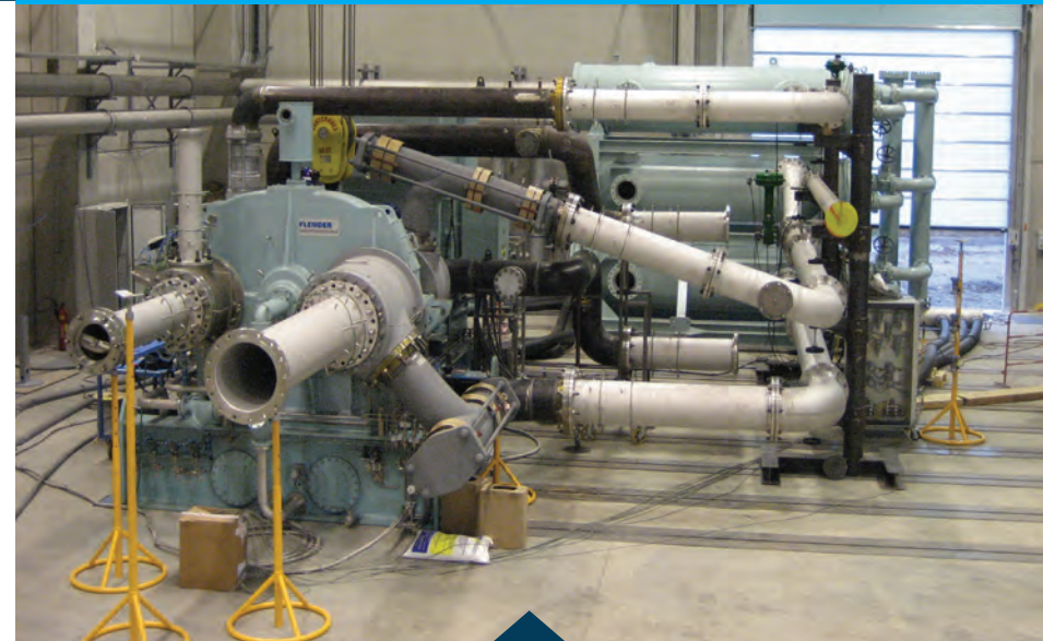
Compander during final test in CRYOSTAR test bench hall
